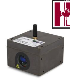
The FlatMesh Optical Displacement Sensor Node is an instrument which uses optical means to take high precision displacement measurements and pass these through Senceive's FlatMesh wireless communications network to a FlatMesh Gateway. It can also be combined with Senceive's world-leading triaxial tilt sensor to obtain high precision tilt measurements that are linked to an external reference.
